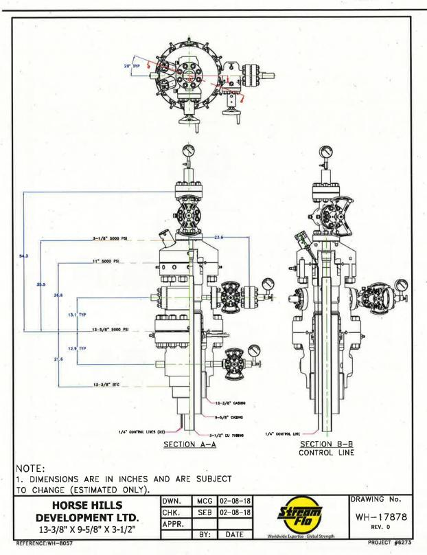
Proposed wellhead arrangement with 3 1/2" tubing hanger
