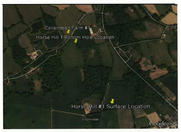
The bottom hole location which is marked is at the TD of the original borehole at 8,815 ft MDBRT
