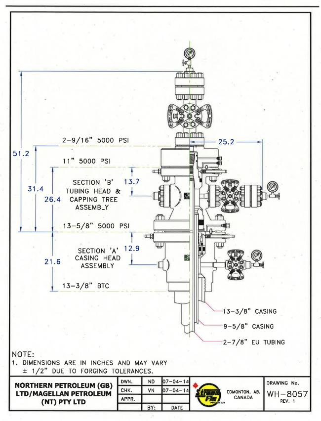
Current wellhead arrangement with 2 7/8" tubing hanger
